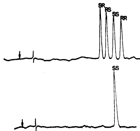
Figure 2. HPLC chromatograms of [ phenoxyphenyl - ^{14}\text{C} ]fenvalerate and the resolved [ ^{14}\text{C} ] SS isomer. The HPLC retention times for the SR , RS , SS , and RR isomers are 20.5, 22.1, 24.0, and 26.1 min, respectively (flow rate 1 mL/min).
